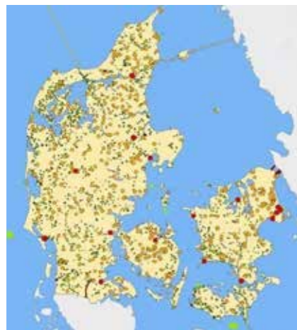
CHP and wind development in Denmark from 1985 (top) to 2009 (bottom) as a result of strong national policies for renewables and district heating. The maps show centralized (red circles) and decentralized (orange circles) CHP plants, onshore and offshore wind power (green circles) and interconnectors (Lauersen, 2014).
