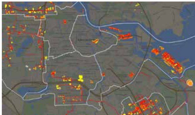
City of Amsterdam, Interactive Maps , 'Energy from waste incineration and waste heat'. Map showing the existing district heat network in Amsterdam (red) with connected load (yellow) and sources of waste heat (orange).
